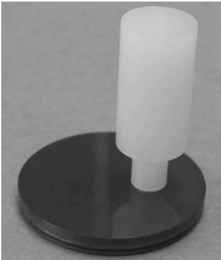
Figure 1. The pin and disk configuration for articulation.
