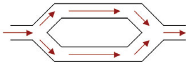
Figure 1. Schematic of a Mach Zender interferometer consisting of a polymeric waveguide with two optical paths. The laser beam enters from the left and leaves to the right
