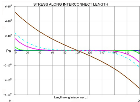
(b) interface treated like a free surface of Cu
