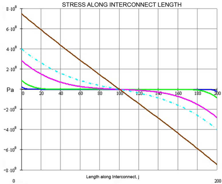
Figure 6.4: Curves of calculated stress evolution in an interconnect line (at T= 573\text{K} and times of 30, 6, 3, 0.3 and 0.03 hours (no change) at a current density of 25 mA per square micron). The interface is treated like a free surface of Cu and the interconnect has no overhang length. Peak stress reached is 750 MPa.
