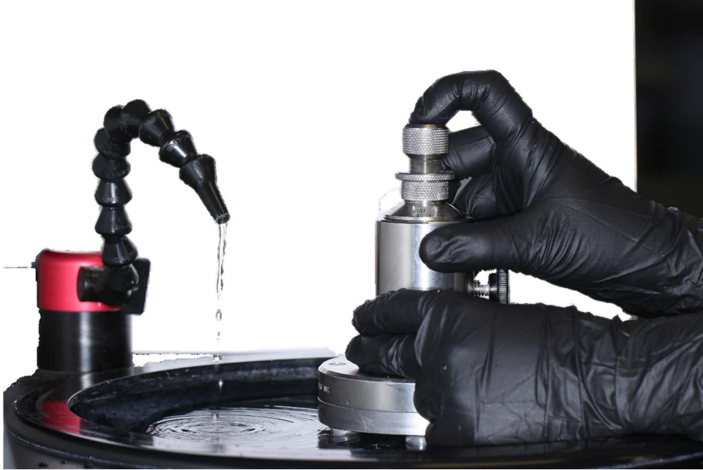
Figure 2: Polishing under water lubrication
