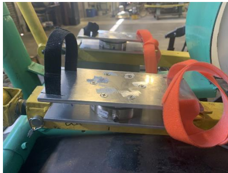
Figure 12. The load cells sandwiched between two plates.
