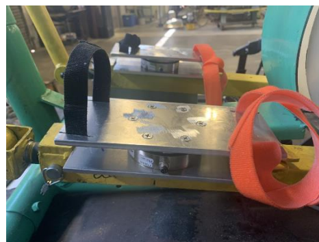
Figure 12. The load cells sandwiched between two plates.
