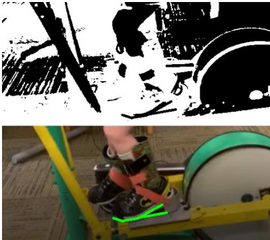
Figure 10. Hough Transform creating black/white image for edge extraction and angle estimation.
