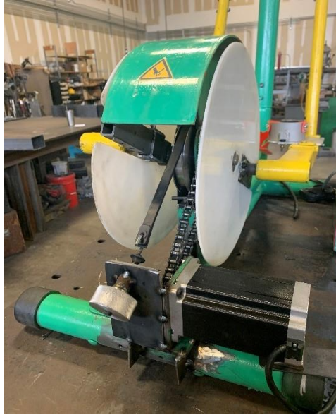
Figure 7. The new design concept with the bicycle freewheel sprocket.
