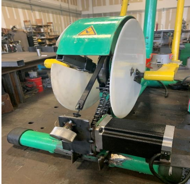
Figure 7. The new design concept with the bicycle freewheel sprocket.
