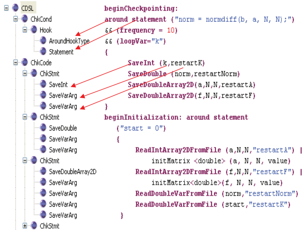
Figure 3-21- DSL code mapped into KM3 model
