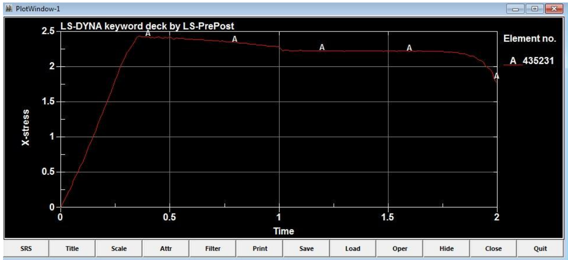
Figure 99: Time-stress graph of rectangular – 6 inch concrete barrier element in tension side with maximum stress
