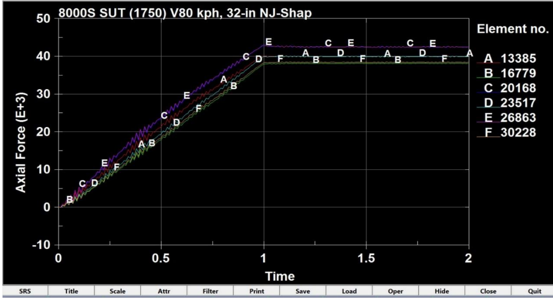
Figure 78: Time-Axial Force Graph of New Jersey barrier hairpin dowel reinforcement bar element in tension side with maximum stress
