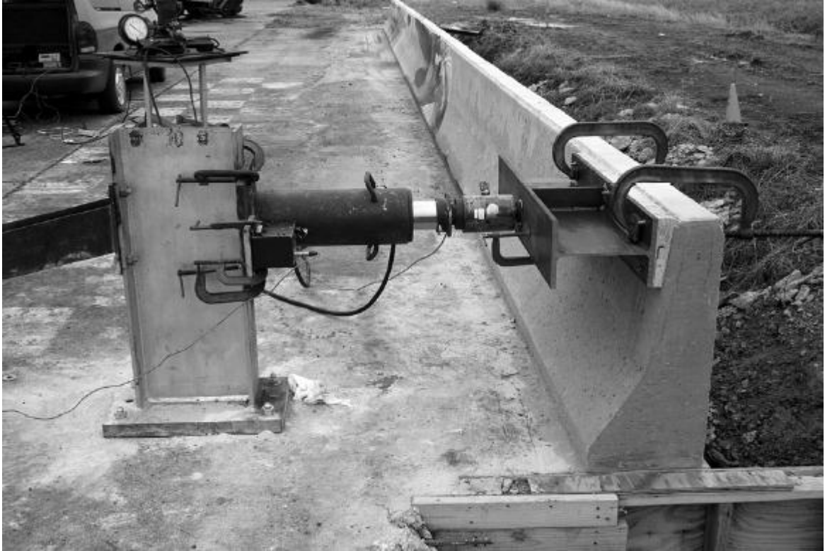
Figure 56: Static Load Test Setup for Safety-Shaped Barrier (After Abu-Odeh, Bligh, & Yvonne, 2007)
