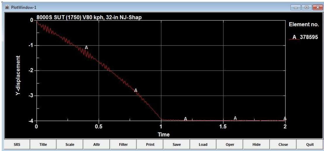
Figure 135: Maximum Deflection of the New Jersey Barrier
