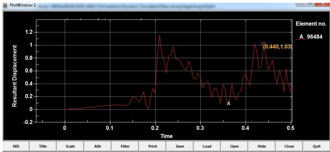
Figure 259: Maximum deflection of the deck overhang at second impact – New Jersey geometry
