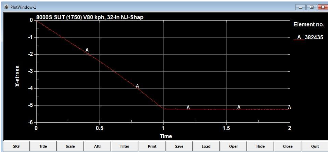
Figure 71: Time-stress graph of New Jersey concrete barrier element in compression side with maximum stress
