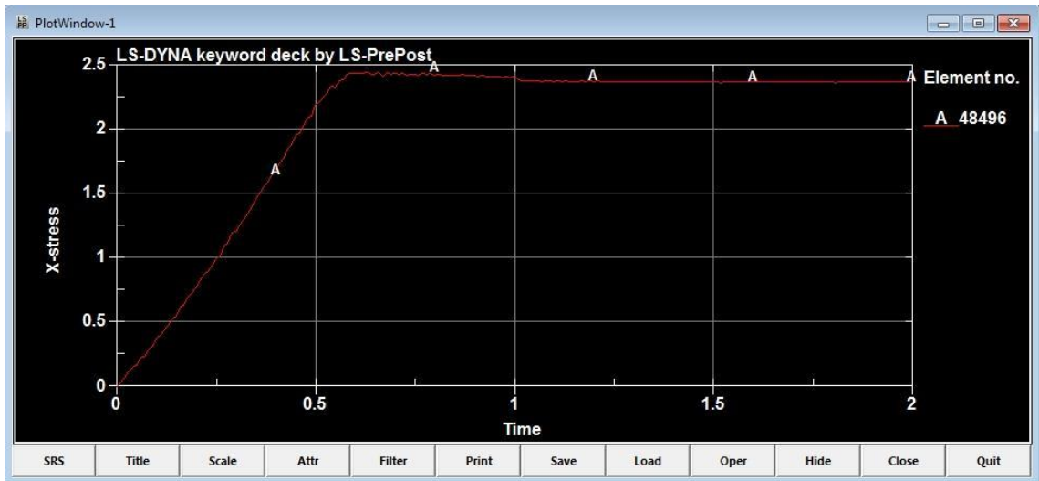
Figure 90: Time-stress graph of rectangular – 8 inch concrete barrier element in tension side with maximum stress
