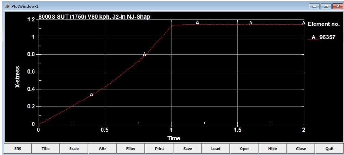
Figure 76: Time-stress graph of New Jersey concrete deck overhang element in tension side with maximum stress
