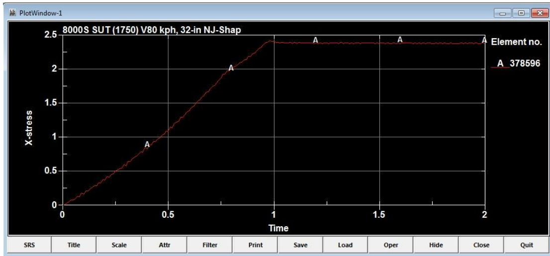
Figure 72: Time-stress graph of New Jersey concrete barrier element in tension side with maximum stress
