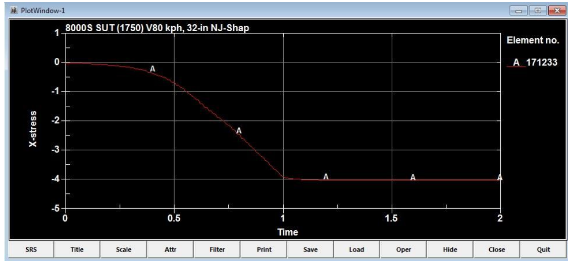
Figure 75: Time-stress graph of New Jersey concrete deck overhang element in compression side with maximum stress
