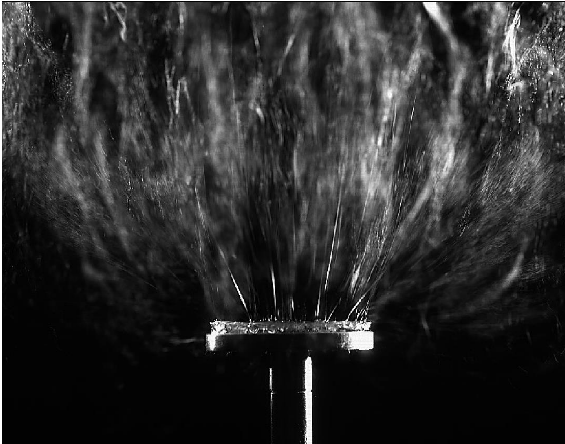
Figure 6. Highspeed electrode comparison. A frame taken from highspeed video of the electrodynamic spinning process. The video was recorded at 2,000 frames per second.
