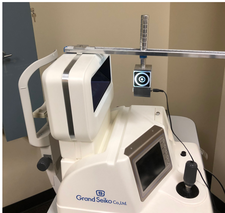
Figure 2: Grand Seiko WAM 5500 with UC-Cube mounted to instrument
