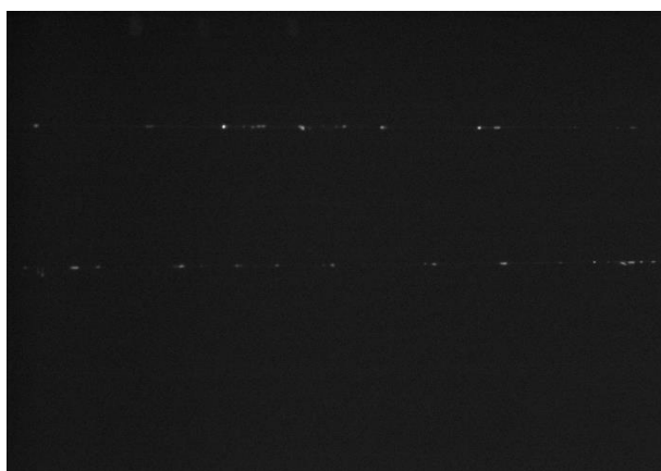
Figure 5. Fluorescent micrograph showing two electrospun PCL nanofibers with fluorescent strain markers adhered along the length of the fiber.
