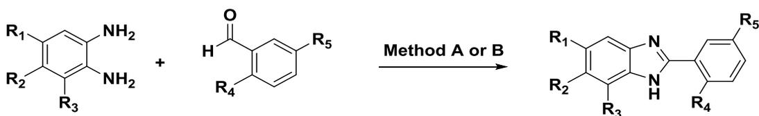
Method A: NaHSO<sub>3</sub>, DMSO, 210°C, 1h; Method B: Na<sub>2</sub>S<sub>2</sub>O<sub>5</sub>. DMF, 170°C, 15 min, MW
