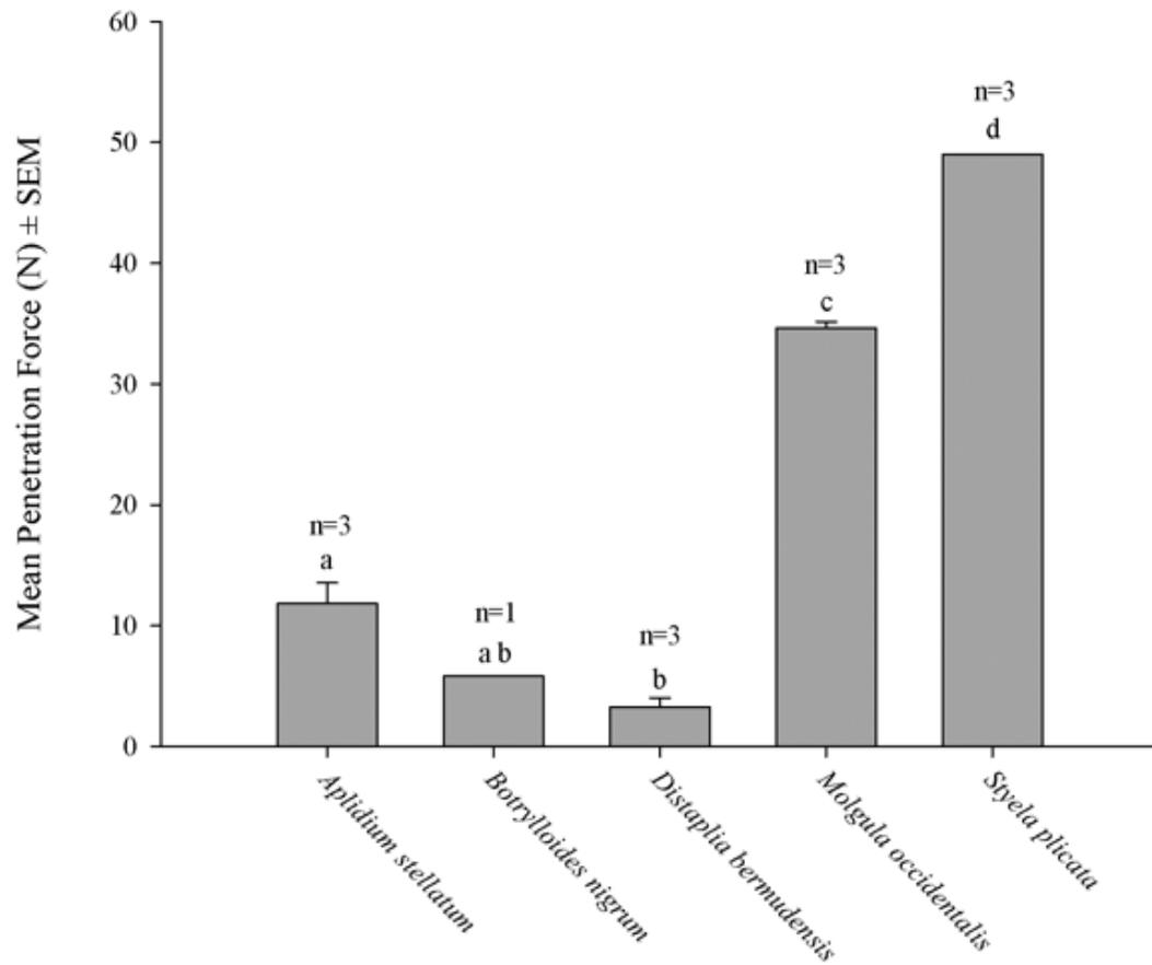
Figure 2. Mean + 1 SE of force required to penetrate the tunic of five species of ascidians. Bars with different letters are significantly different from one another (ANOVA;  $p \leq 0.001$ ). n is given above each bar.
