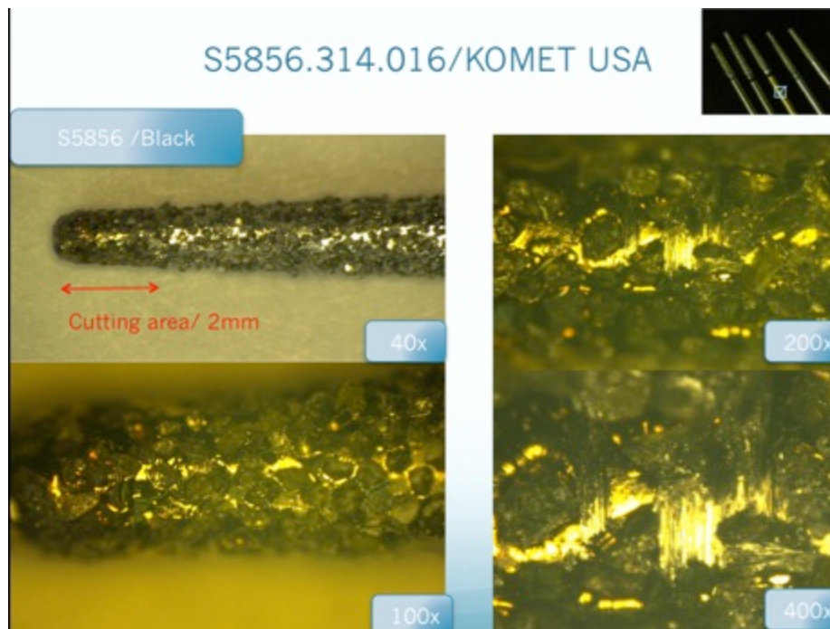
Figure 24: Group8 diamond wear after second cut.
