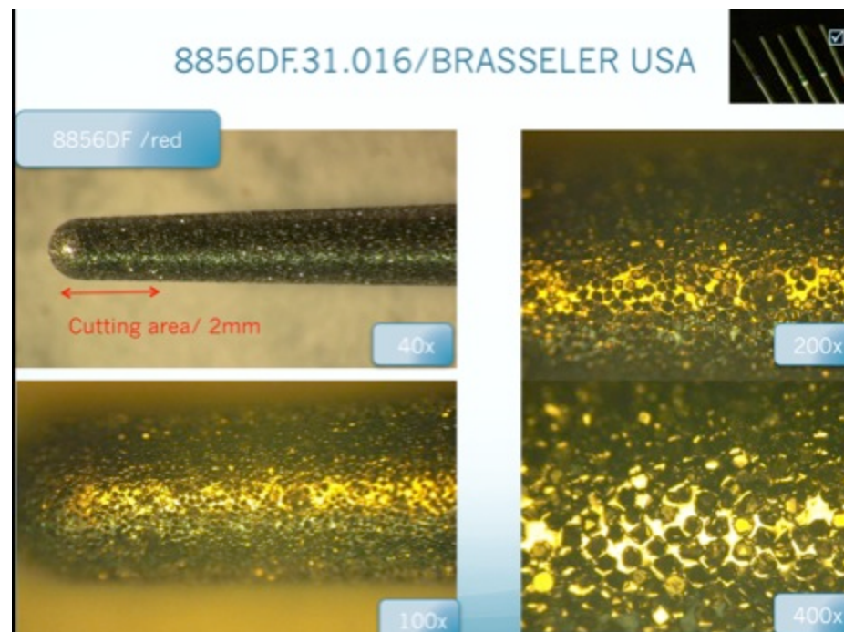
Figure 18: Group2 diamond wear after second cut.
