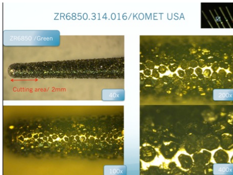
Figure 20: Grou4 diamond wear after second cut.
