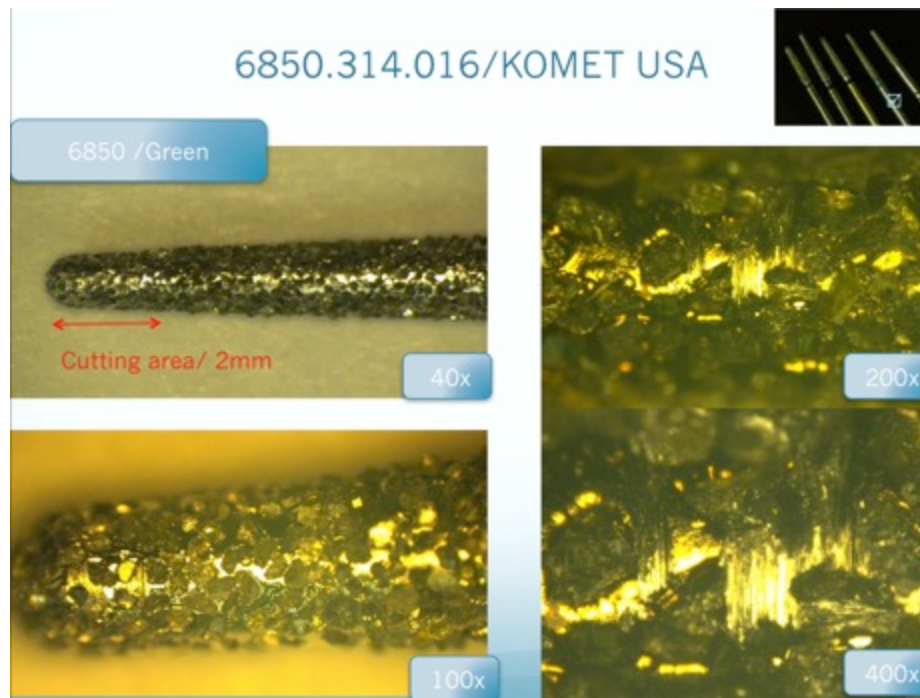
Figure 25: Group9 diamond wear after second cut.
