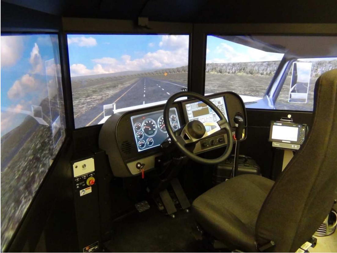
Figure 4. L-3 Communications Truck Driving Simulator
