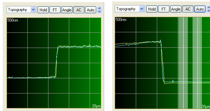
Figure 3-3. Topography by AFM; sample (left) indicates 1020nm while sample (right) shows 1305 nm (each grid has 500nm division)
