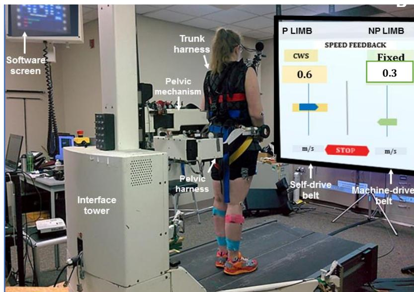
Figure 1B: Poststroke participant standing inside KineAssist (KA) split-belt treadmill interface. For Condition 2: Paretic (P) limb belt (left) was driven by participant (SD) with target CWS speed of 0.6 m/s (yellow zone); while the nonparetic (NP) limb belt (left) was fixed to move automatically (MD) at 0.3 m/s. Vice-versa for condition 2.
