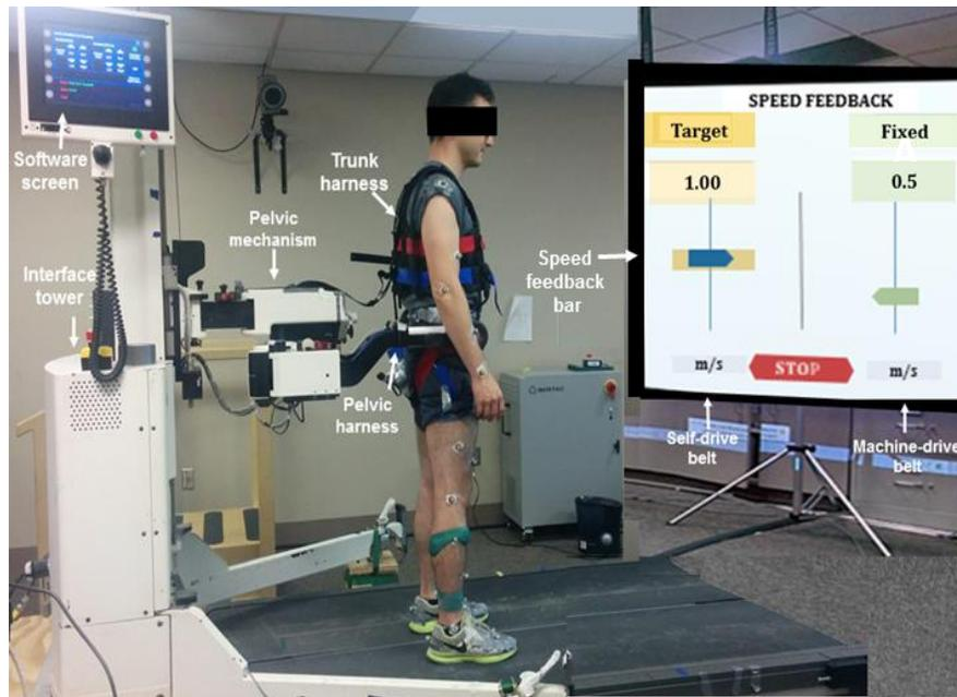
Figure 1A: Nonimpaired participant standing inside KineAssist (KA) split-belt treadmill interface. For experiment 1: Left belt was driven by participant (SD) with target speed of 1 m/s (yellow zone); right belt was fixed to move automatically (MD) at 0.5 m/s. Vice-versa for experiment 2.
