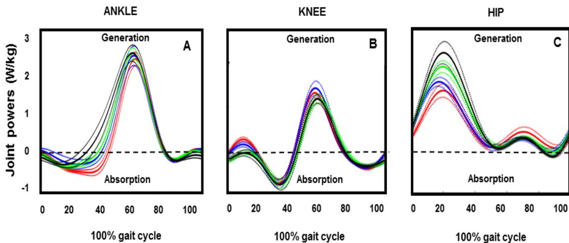
Figure 4. Ensemble average profiles of joint powers with standard error (dotted colored lines) for ankle (A), knee (B), and hip (C), respectively, at 10% (red), 15% (blue), 20% (green) and 25% (black) fore-aft (FA) resistance across 100% of the gait cycle
