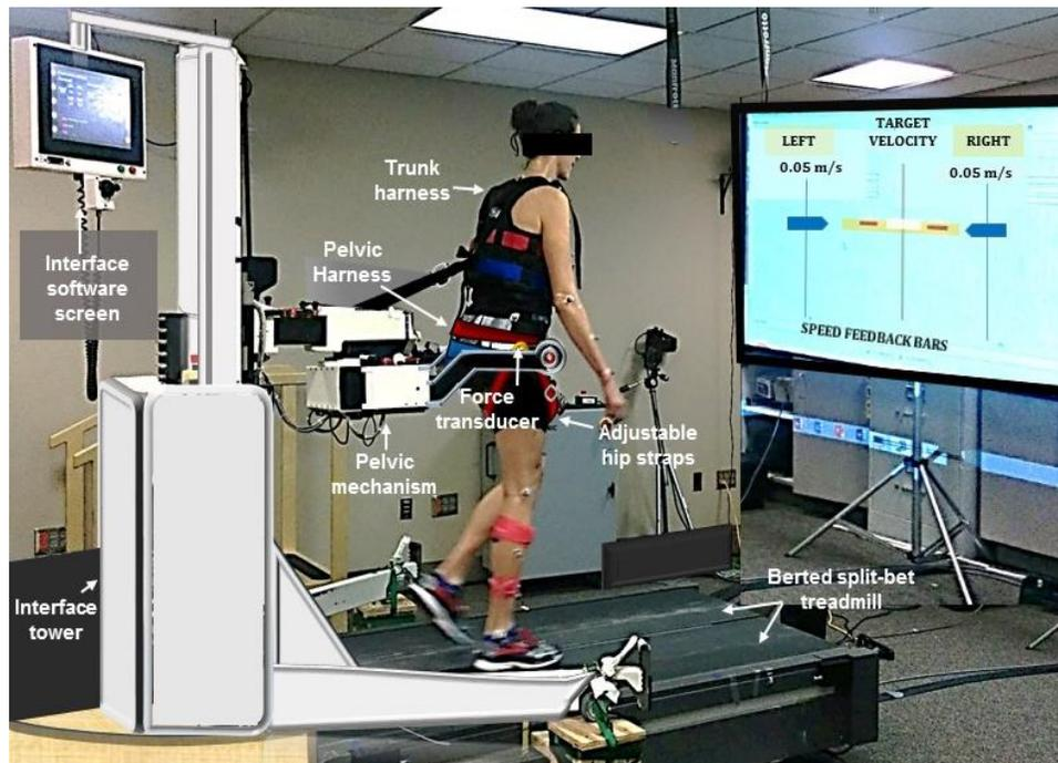
Figure 1: Nonimpaired individual walking inside the KineAssist (KA) robotic split-belt interface targeting a velocity of  $0.5 \text{ m/s} \pm 0.1$  using real-time visual feedback *Note: Tied belt velocity displayed as white bar on yellow target zone*
