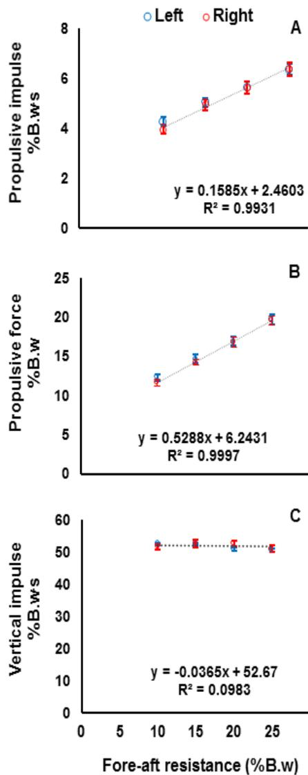
Figure 3: Mean propulsive impulse, propulsive force and vertical impulse with standard error bars (A) propulsive impulse and (B) mean propulsive force (both during 50 to 100% stance), and (C) vertical impulse (during 0 to 100% stance) for each fore-aft resistance trial normalized to body weight
