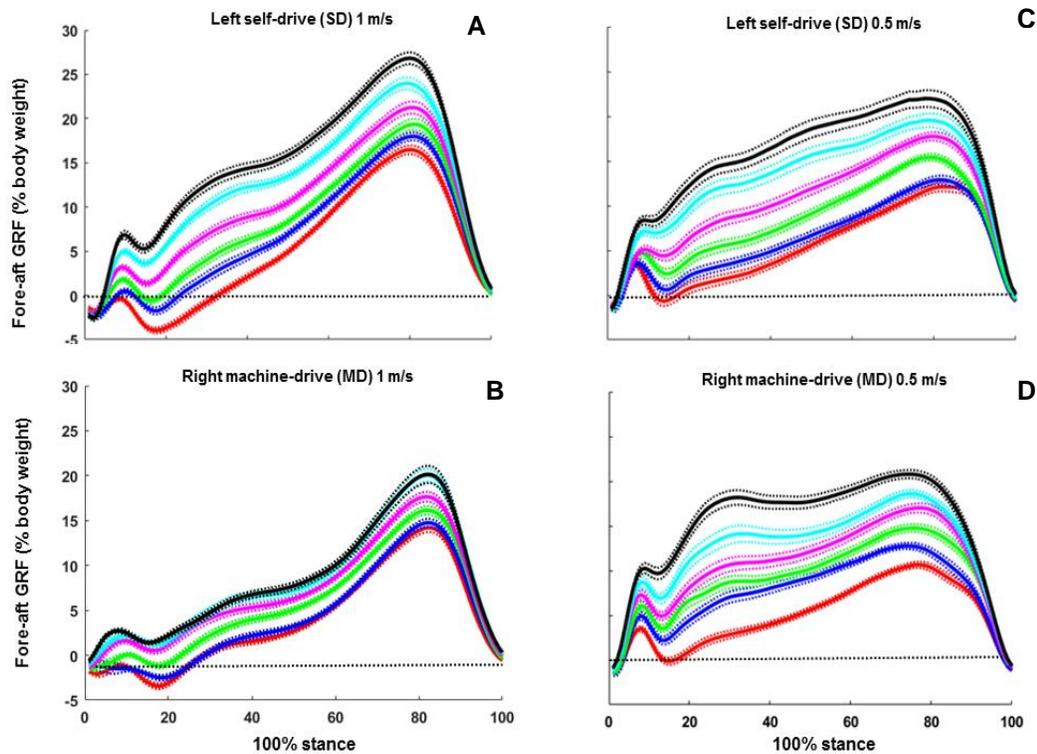
Figure. 2. Ensemble (average with standard error) fore-aft GRF profiles during condition 1 and condition 2 for left self-drive (SD) belt at 1 m/s (Fig.2.A) and right machine-drive (MD) belt at 1 m/s (Fig.2.B) with 0.5 m/s SD (Fig 2.C) and 0.5 m/s MD (Fig 2.D) across all FA resistance conditions. FA resistance levels – 6% (red), 9% (dark blue), 12% (green), 15% (magenta), 18% (light blue), and 21% (black).
