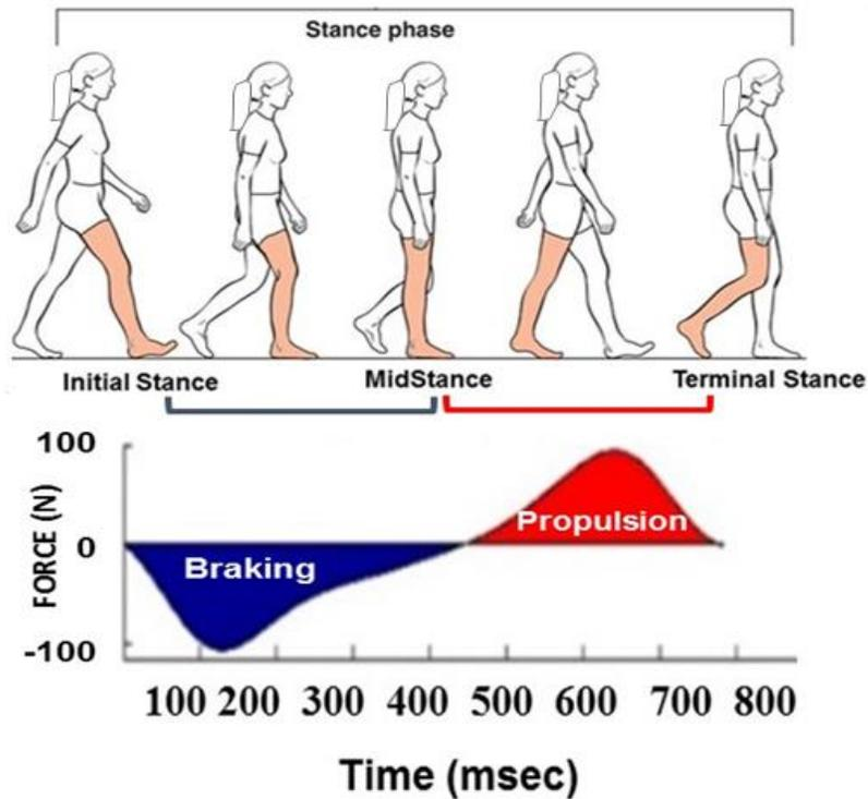
**Fig.2:** Force by time plot for generation of fore-aft (braking and propulsion) ground reaction forces during the stance phase of walking
