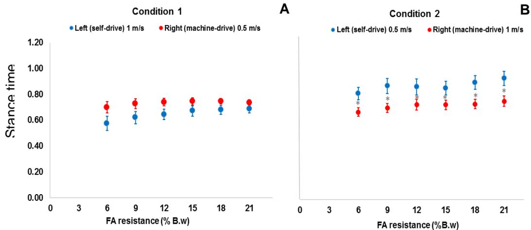
Figure 6: Mean stance time (seconds) with standard error bars for the self-drive (SD) and machine-drive (MD) limbs in condition 1 (Fig.6.A) and condition 2 (Fig.6.B) across all differential FA resistance levels. Note: Grey \* represent significant pairwise comparisons using independent samples *t*-test at  $p < 0.05$ .
