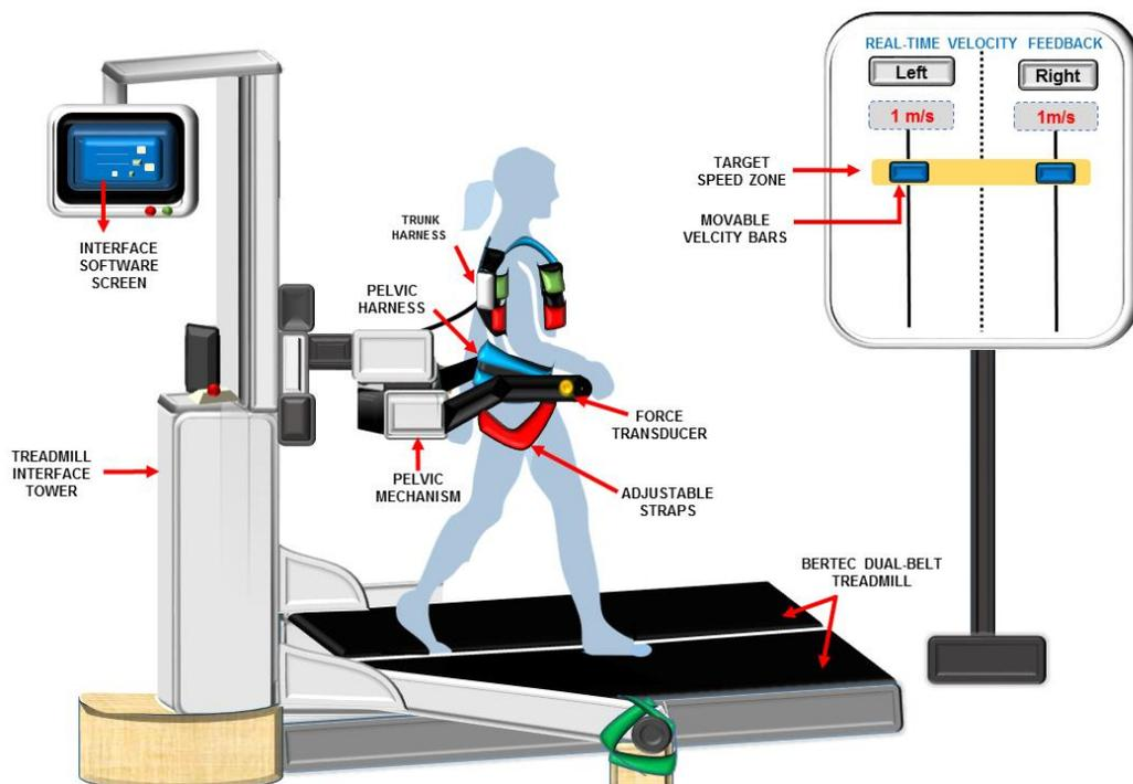
Figure 1: Participants walking inside the KineAssist (KA) split-belt treadmill interface using visual feedback via the interface's software output to target  $1.0 \pm 0.2$  m/s highlighted by a yellow target zone and, projected on a screen (at eye level)
