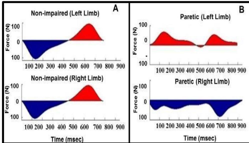
Fig.3 (A). Fore-aft ground reaction force for a single step of a non-impaired individual (A) walking at a constant speed with symmetric braking (Blue) and propulsion (Red) forces. An individual poststroke (B), walks with increased paretic braking force (Blue) and greater non-paretic limb propulsion for a single step at comfortable walking speed (Red).
