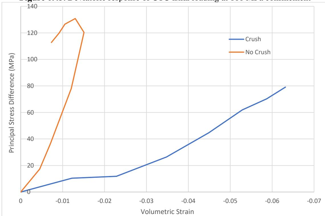
**Figure 0.46:** Volumetric response of CTC axial loading at 100 MPa confinement
