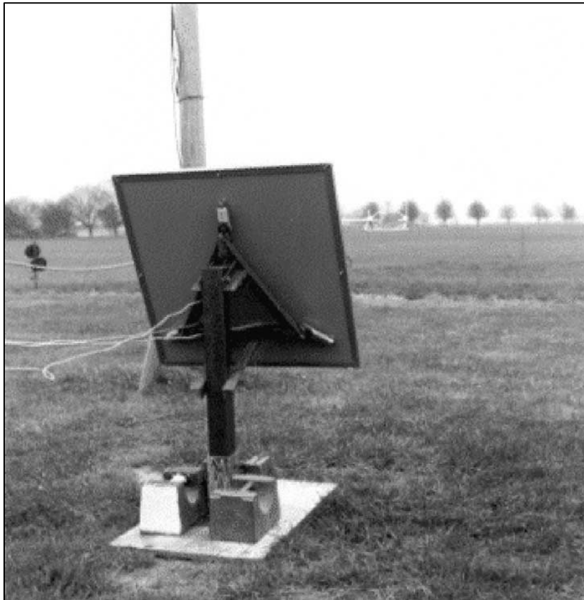
Figure 2-7: Photo of 750 mm square sign mounted on support frame (Quinn 2001)
