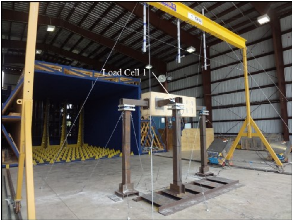
Figure 3-3: Tare test Setup A for 0° configuration (Meyer 2014)
