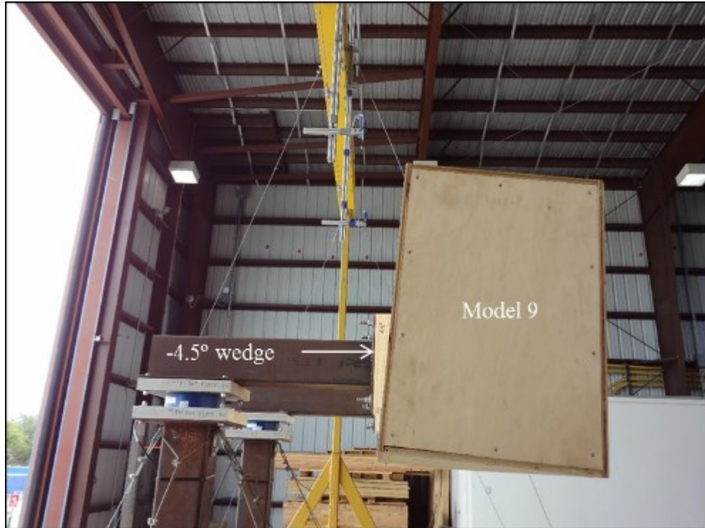
Figure 3-8: Galloping test setup for -4.5^\circ angle (Meyer 2014)
