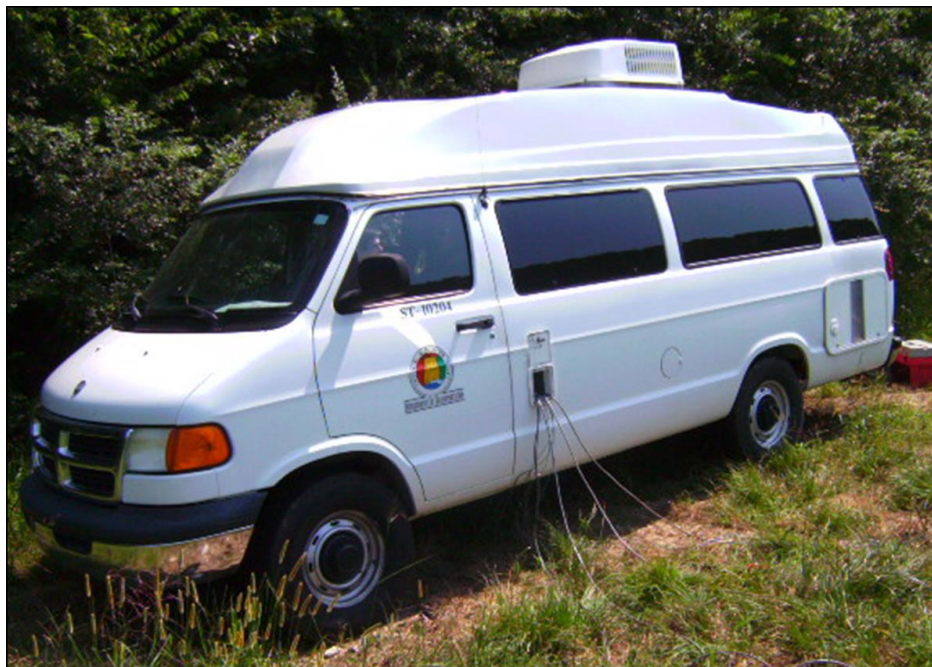
Figure 6-10: ALDOT Van with Instrumentation Wiring (Fouad 2011)
