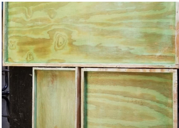
Figure 13. Wood molds used for casting platforms of syntactic foam.
