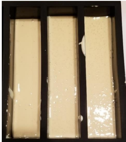
Figure 9. Three samples of syntactic foam used for four-point bending tests.
