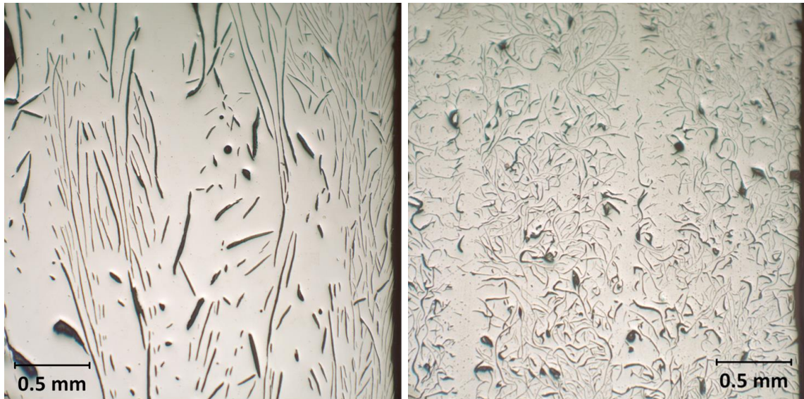
Gray iron alloy #1 (4.36%CE, 1.5%Si) at 1µm/s
