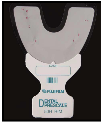
Figure 12. Pressure indicating film that is used to measure biting forces
