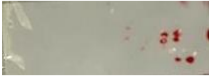
Figure 37. Change in Prescale film color after biting
