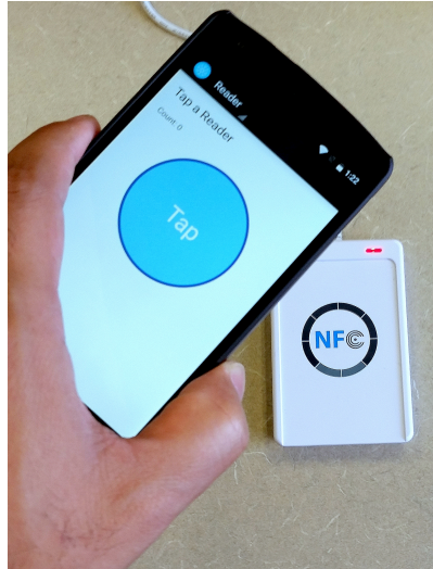
FIGURE 5.4: A user tapping an NFC reader at waist-flat position. In waist-flat scenario, the NFC reader is kept at the height of 0.75-1 m from the ground and horizontally on the table.
