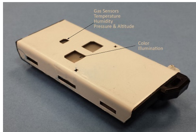
FIGURE 6.1: Sensordrone device with different sensors (ambient temperature, precision gas, humidity and altitude are utilized in this work). Device dimensions: 2.67 x 1.10 x 0.49 inch 3 .
