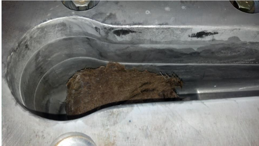
Figure 45. Extruded charge placed 25.4 mm away from the female tool radius end.
