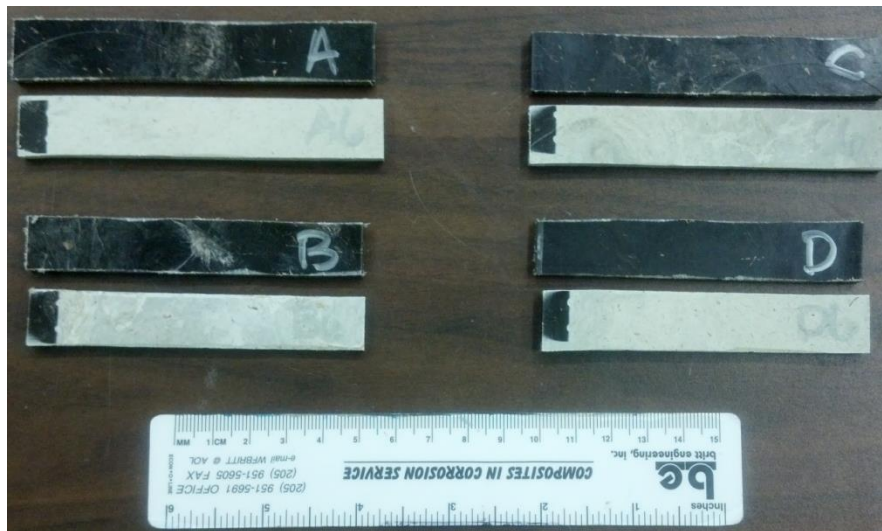
Figure 39. Flexural samples exposed to UV radiation for 1,000 hours.
