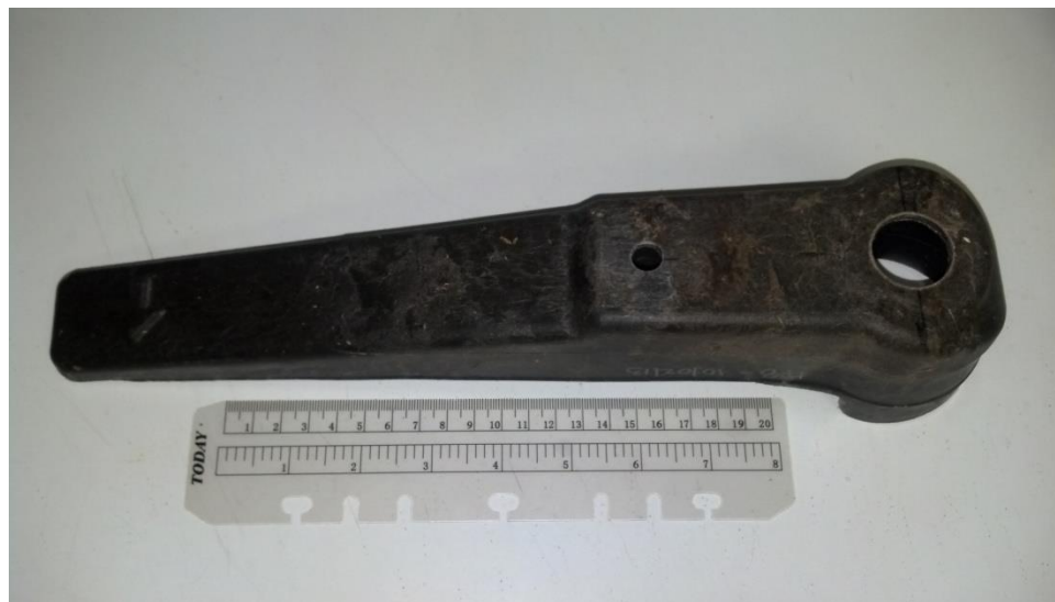
Figure 46. 30 wt. % hemp fiber reinforced PP composite with 5 wt. % MAPP duct-screen prototype via compounding-extrusion-compression molding manufacturing process.
