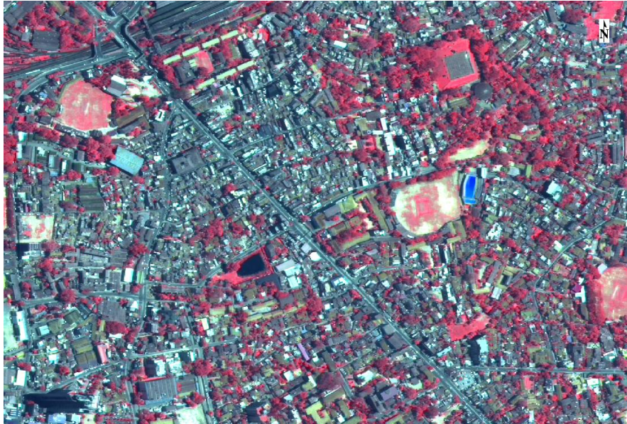
Figure 4: Quickbird false color composite consisting of NIR, Red, and Green bands as red, green and blue; Courtesy: DigitalGlobe Inc.
