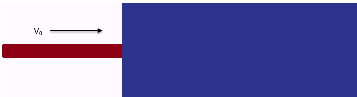
Figure 5.11: Initial conditions for penetration of an L/D=10 tungsten rod into a semi-infinite steel target.
