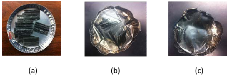
Figure 4. (a) Carbon fiber thermoplastic composite sample with known nominal fiber content before carbonization; (b) residue from composite sample after CIN; (c) residue from the reference neat resin after CIN.
