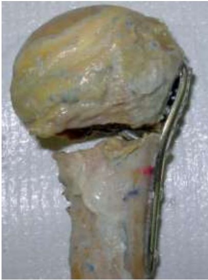
Figure 24: Mode of failure in medial comminuted specimens. Before loading (left) and after loading (right)
