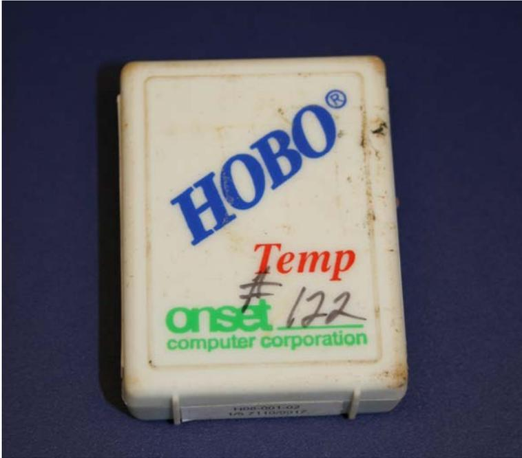
Figure 2. A HOBO temperature data logger like those used in the nest temperature project for Juno Beach, Florida.
