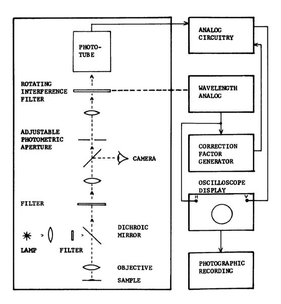
instrumentation to produce corrected fluorescence emission spectra on-line. The light microscope is a Leitz Orthoplan equipped with a Ploem type epi-illumination system which is normally used for fluorescence measurements, and a transmitted light Smith interference contrast imaging system. The latter system is not shown in the diagram.
